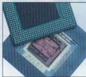
The Emotion Engine and Graphics Synth (above) are finished chips (which require a hefty amount of cooling during operation – see right) but the NGPS's internal architecture is still in the process of being tweaked
